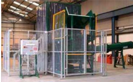
Complete revolution™ 2000 series system installation with control panel, safety guarding, pallet tipper and lift equipment
