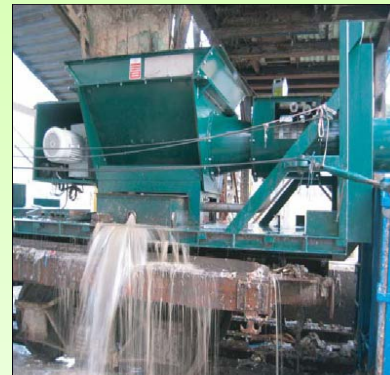
revolution™ 2000 series removing liquids from re-pulping waste stream
